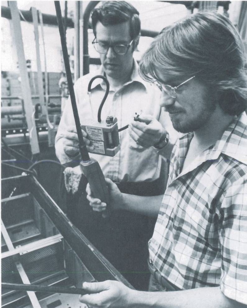
ENVIRONMENTAL TESTING: Bill Dudley, safety coordinator at the New Jersey Division, collects samples of methylene chloride fumes from a vapor degreaser in Gary Martinsen's work area.
